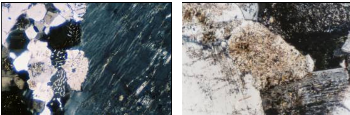
Figure 32 - Microscopic observations (N+; magnification x70) of pinkish granite samples: myrmekitic texture (left) and plagioclase altered to sericite and occasionally to calcite and epidote (right).
