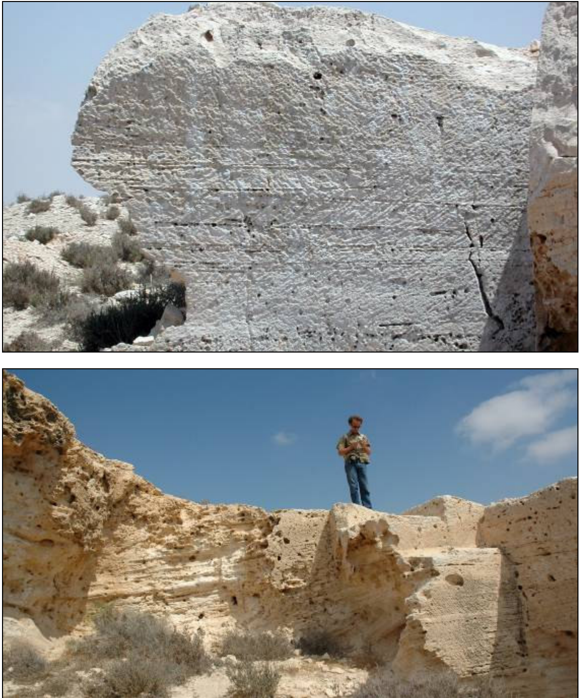
Figure 105 – Views of the main quarry of Abu Sir area: beige porous calcarenite limestone with (up) typical cross-bedding and (down) intense weathering form (alveolisation).
