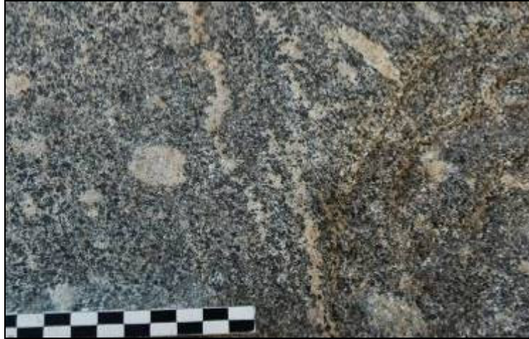
Figure 33 – Representative megascopic view of a dark-grey granodiorite sample: porphyritic texture with pluricentimetric white-milk plagioclase phenocrysts.
