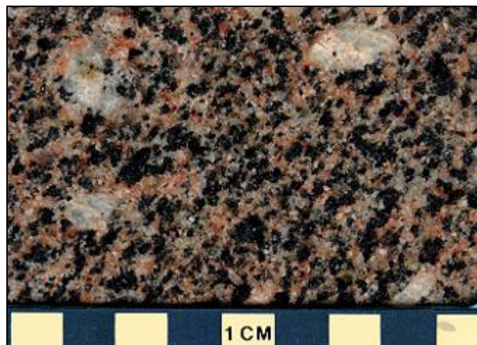
Figure 61 - Megascopic view of type (c) Aswan granitoid (from J.A. Harrel, modified, http://www.eeescience.utoledo.edu/Faculty/Harrell/Egypt/Quarries/Quarries_Menu.html ).
