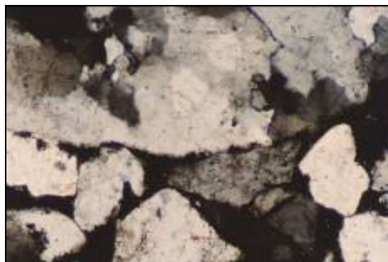
Figure 88 - Microscopic observation (N+; magnification x110) of silicified sandstone sample (A125 = unfinished obelisk) from Gebel Gulab: orthoquartzite with interlocked grains slightly silicified.
