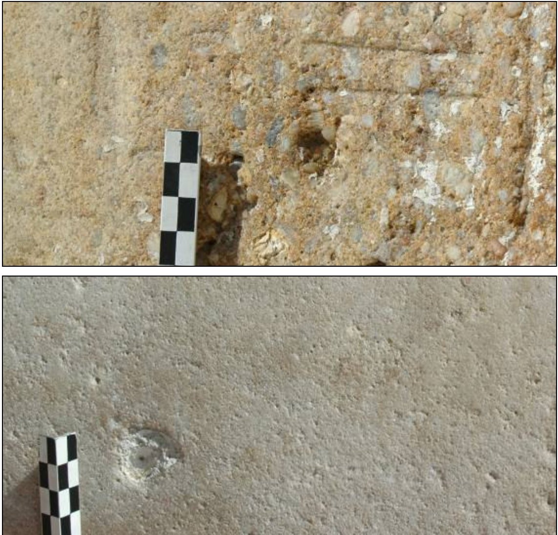
Figure 40 - Megascopic views of siliceous sandstone objects: (up) beige-yellowish to ochre coarse-grained (almost conglomeratic) siliceous sandstone (sample A10); (down) beige fine-grained siliceous sandstone (sample A12).
