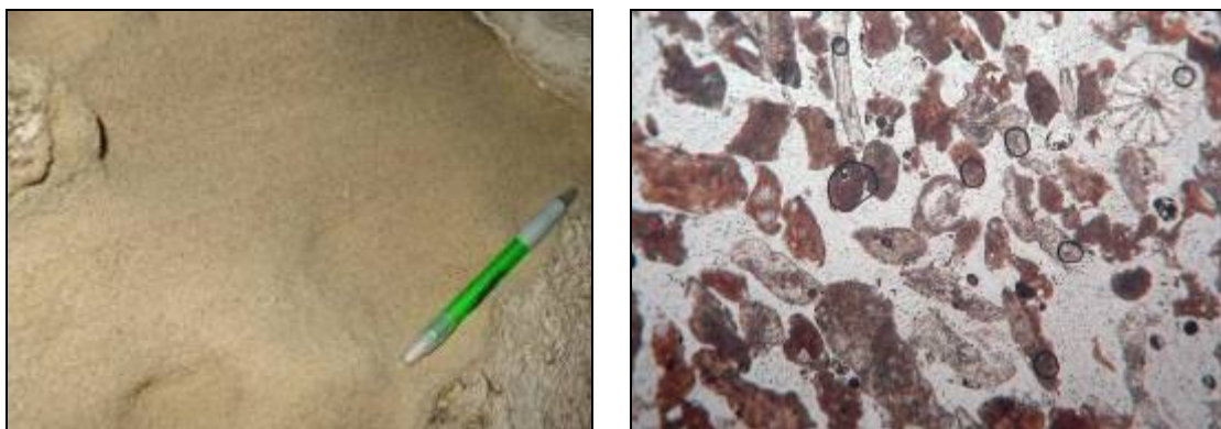
Figure 55 – Megascopic (left) and microscopic view (N//) of the bedrock of Qaitbay Fortress (sample A5): light beige-grey calcarenite sandy in texture and very friable.
